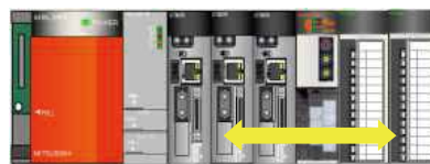
Direct control between CPUs and I/O units
